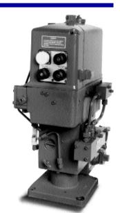
PGG governor/actuators are available with any of the PG output systems. Output ranges from 16 N·m (12 lb-ft) maximum work capacity to 678 N·m (500 lb-ft), depending on the governor operating pressure and the output options selected. Most outputs provide 30° of rotary travel (25 mm [1 inch] of linear travel is also available).
