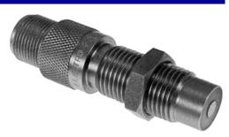
When a magnetic material (usually a gear tooth driven by the prime mover) passes through the magnetic field at the end of the magnetic pickup, a voltage is developed. The frequency of this voltage is translated by the speed control into a signal which accurately depicts the speed of the prime mover.
